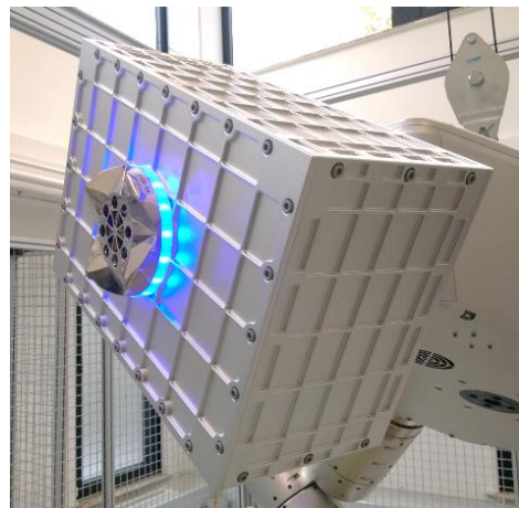
Figure 27: MIRROR's ORU connected to the MAR's leg.
