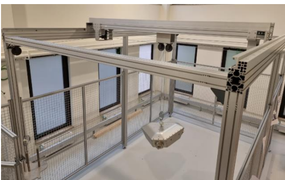
Figure 25: Offloaded MAR's torso.
