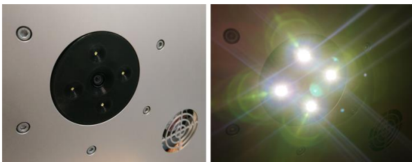
Figure 19: Torso's vision subsystem: lighting module off (left) / on (right).
